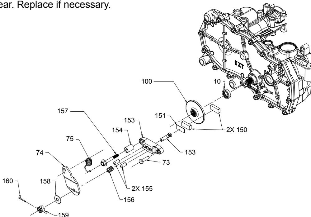
Figure 9. Disc Brake Assembly
