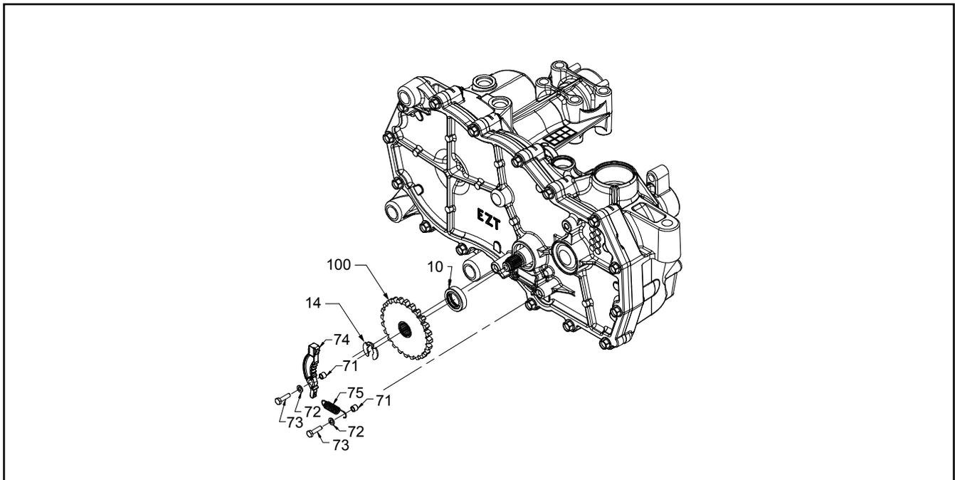
Figure 8. Cog Brake Assembly
