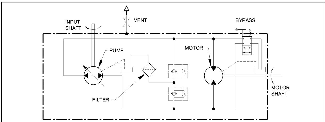
Figure 1. Hydraulic Schematic
