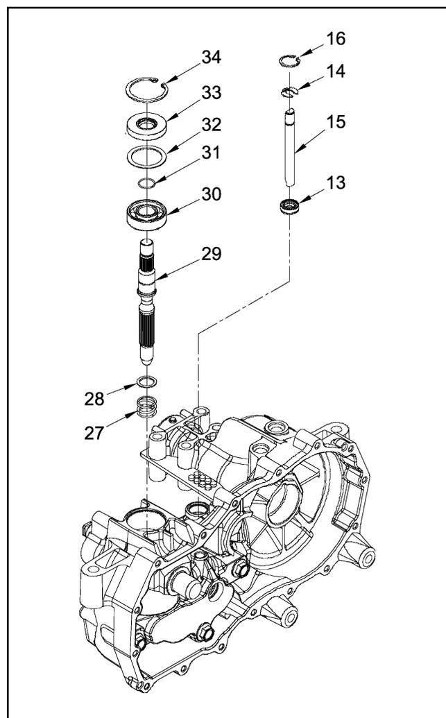
Figure 13. Input Shaft and Bypass Rod Assembly
